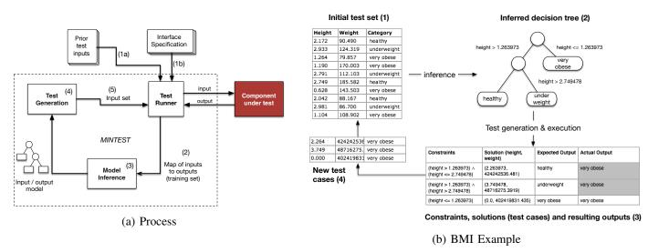
Fig. 1. Inference-driven test generation process
