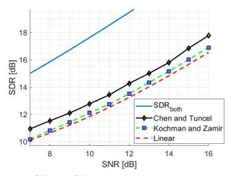
Fig. 2: SDR vs SNR for the model in Sec. III with  $\sigma_Z^2 = 1/9$ . "Chen–Tuncel" and "Kochman–Zamir" are the schemes from [13], [15] with parameters  $(\Delta, \alpha, \beta) = (3.15, 0.8, -1.15), (2.15, 1.05, 0)$ , respectively.
