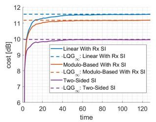
Fig. 3: Control cost evolution across time for Schs. 3–5 for SNR = 6dB,  $\sigma_W^2 = 1$ ,  $\sigma_Z^2 = 1/8$ ,  $\lambda = 2$ , Q = 5, R = 1. The parameters used in Sch. 5 for transmission are  $\alpha = 0.75$ ,  $\beta = -1.18$ ,  $\Delta = 3.2$ . The plots are averaged over  $2^{10}$  runs.
