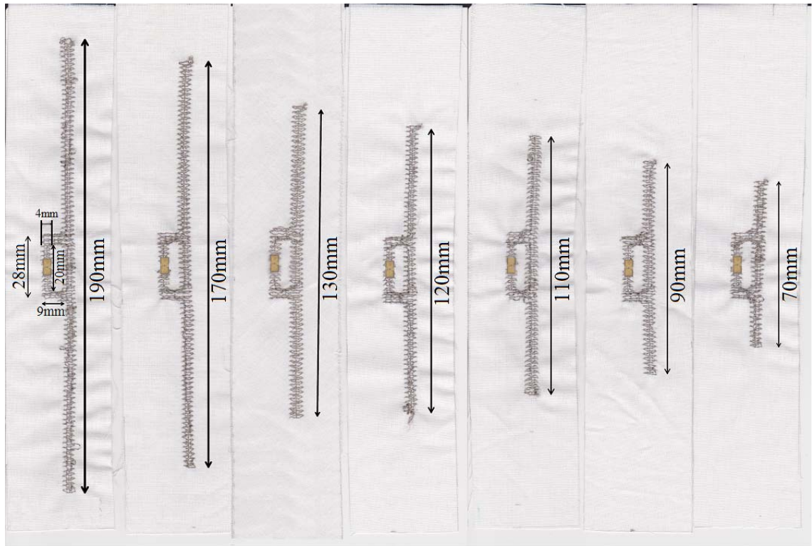
Figure 7.5. Sewed antennas with the same T-match geometrias before, but with different lengths.
