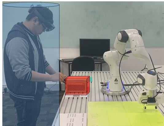
Fig. 1: A user, wearing an augmented reality headset, is shown collaborating with the robot using our Virtual Barrier system. Using our system, users can collaborate with the robot while being protected by a Virtual Person Barrier (blue cylinder). Objects in the shared workspace can be protected by Virtual Obstacle Barriers (red rectangular prism).
