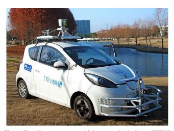
Fig. 1: Tongji autonomous vehicle research platform "TIEV"
