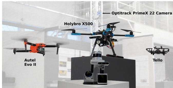
Fig. 1: Illustration of the hardware used in the experiments. At the bottom, the tracking sensors including Ouster OS1-64, Livox Mid-360, Livox Avia and Intel RealSense D435.
