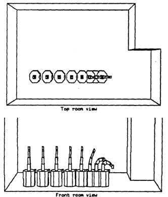
Figure 7: Simulation 4: Movement with distancedependent artificial damping functions
