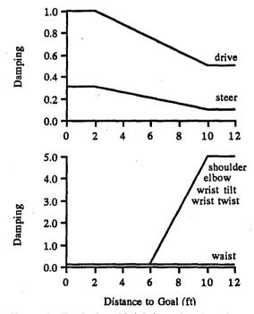
Figure 2: Typical artificial damping functions
