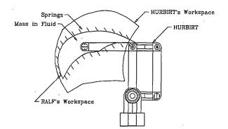
Figure 2: Virtual walls for bilateral teleoperation
