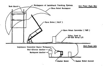
Figure 1: Long-reach teleoperation testbed
