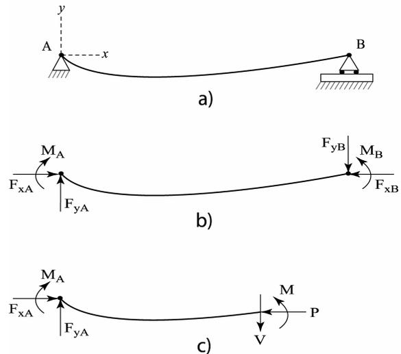
Figure 2 beam derivation diagrams
