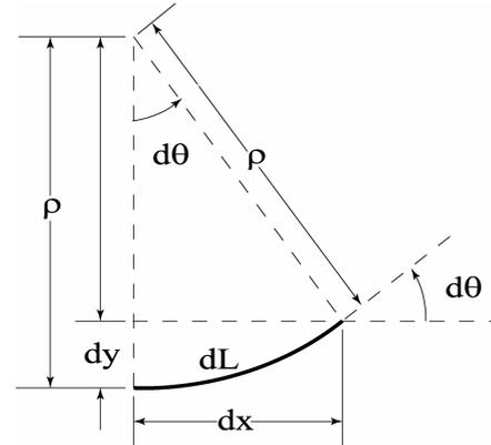
Figure 3. Beam curvature model.
