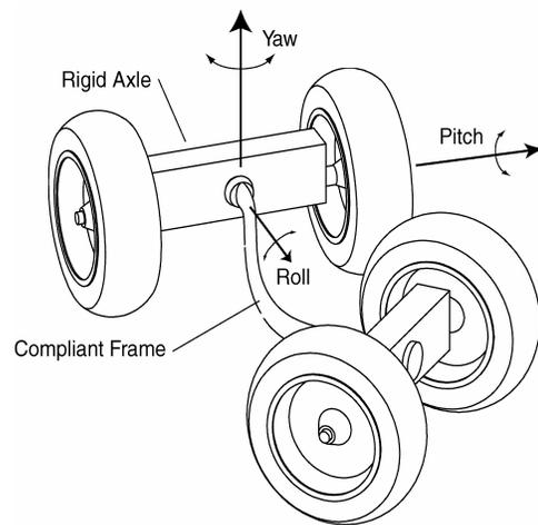
Figure 1. Compliant framed modular mobile robot.
