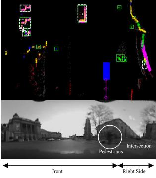
Fig. 5: Pedestrian Detection. The SLAM result shows that the test vehicle was moving at 21.0 mph.
