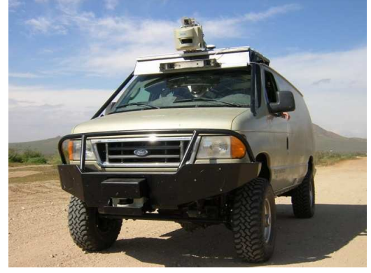
Fig. 2. Our test platform is a 2005 Ford E-350 Econoline van modified by Sportsmobile of Fresno, California. A roof-mounted LADAR and INS provide the raw data used for navigation of desert roads.
