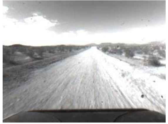
Fig. 4. Visual forward image corresponding to position 2 of Fig. 3. LADAR-based road feature estimation has the advantage of insensitivity to lighting conditions such as long shadows, but is limited to a single lookahead range. Computation times are significantly faster with LADAR feature extraction.
