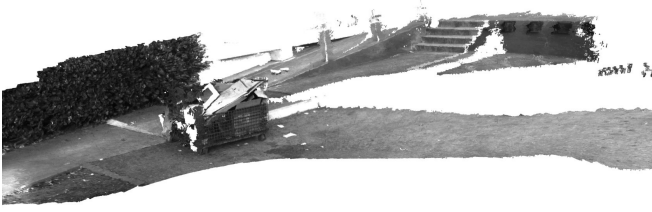
Fig. 5. Globally aligned point cloud model for a dataset composed of approximately 1600 stereo frames.
