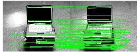
Fig. 4. Example of Sift Output
