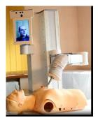
Fig. 2. The ReMeDi system on the site of the patient which shows the robot with an attached screen to display the doctor's face.
