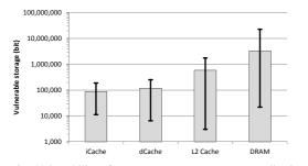
Fig. 6. Vulnerability of memory components across applications
