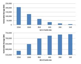
Fig. 7. The impact of L1-Cache resizing on (a) L1-Cache and (b) L2-Cache vulnerabilities
