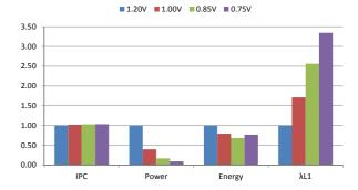
Fig. 10. The impact of VFS on performance, power, energy and L1-Cache reliability, normalized to nominal supply voltage of 1.2V
