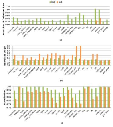
Fig. 13. The impact of L1-Cache resizing on (a) L1-Cache reliability (b) performance and (c) energy; under supply voltage of  $0.85 \mathrm{V}$
