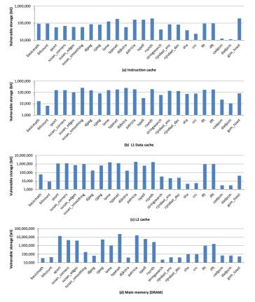
Fig. 5. Vulnerable storage of different memory components for different MiBench benchmark applications: (a) L1 instruction cache (I-Cache), (b) L1 data cache (D-Cache), (c) L2-Cache and (d) DRAM
