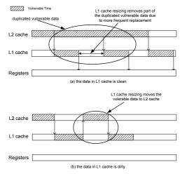
Fig. 8. Vulnerability under L1-Cache resizing when L1-Cache data are (a) clean and (b) dirty
