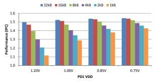
Fig. 11. The impact of L1-Cache resizing on performance under VFS
