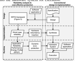
Fig. 9. Proposed reliable design flow
