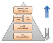
Fig. 1. Microprocessor memory hierarchy
