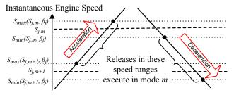
Figure 8: Engine speed range for mode *m* execution
