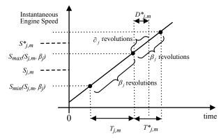
Figure 7: Changes in engine speed over two invocations.
