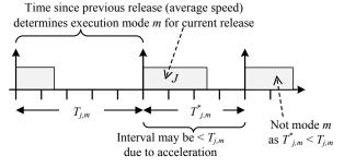
Figure 6: Lag in determining the execution mode
