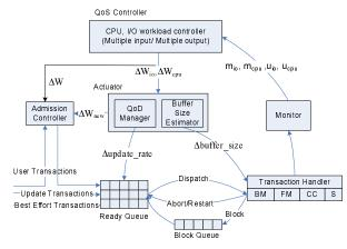
Figure 2: Feedback control architecture
