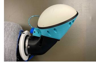
Fig. 6: Our Soft-bubble “paw” module end effectors.
