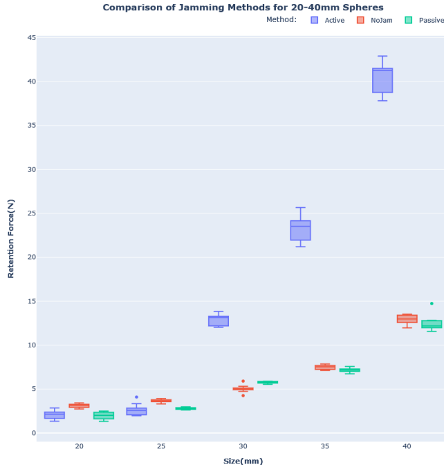
Fig. 6. Boxplot showing increasing grip forces (N) with increasing object size amongst the three gripper configurations tested. Active jamming is seen to have a large impact on grip strength on objects 30mm and over. Bars denote standard error.
