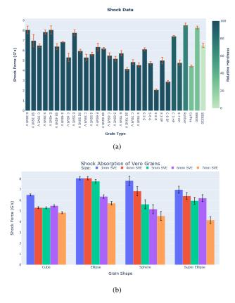
Fig. 6. (a) Shock Absorption properties of each grain type in units of G (lower is better). Bars are coloured according to grain hardness, with darker greens representing harder materials and the lightest green representing a Shore value of 0. (b) Comparison showing the effects of grain size and shape on shock absorbance for 3D printed grains.
