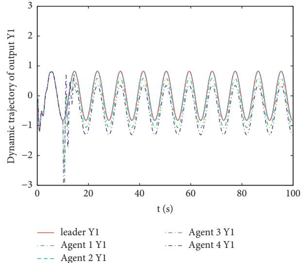
FIGURE 4: Profiles of output trajectories  $y_{i1}$  without fault-tolerant controller.
