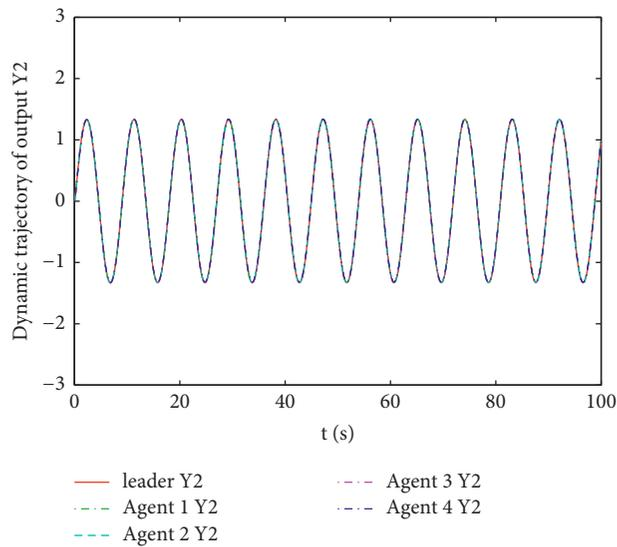
FIGURE 7: Profiles of output trajectories  $y_{i2}$  with fault-tolerant controller.
