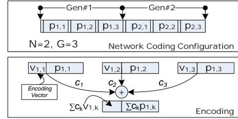
Fig. 1. An illustration of network coding: A file has six  $B$  KB pieces and has configured for coding with the number of generations  $N = 2$  (i.e., the generation size  $G = 3$ ). When GF(256) is used, the size of an encoding vector is 3 bytes (i.e.,  $G$  dimension vector). The bottom figure shows how an encoded piece is created from the first generation.
