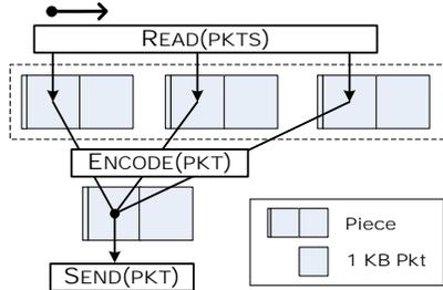
Fig. 3. Overall procedure example:  $G = 3$  (generation size),  $B = 2\text{KB}$  (piece size). A coded piece is composed of 2 independent 1-KB coded packet. Each piece has a header composed of an encoding vector, generation number, etc.
