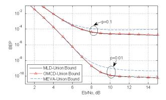
Fig. 2. The union bound on the Bit Error Probability (BEP) of MLD, MEVA and the proposed OMCD for a convolutional coded system under the BG noise model with  $\Gamma = 400$  and  $p = \{0.01, 0.1\}$ .
