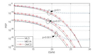
Fig. 4. The pairwise error probability of MLD, MEVA and the proposed method under the BG noise model with  $\Gamma = 100$  and  $p \in \{0.001, 0.01, 0.1\}$ .
