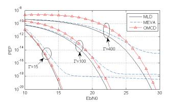
Fig. 3. The pairwise error probability of MLD, MEVA and the proposed method under the BG noise model with  $\Gamma \in \{15, 100, 400\}$  and p = 0.02.
