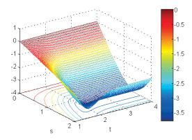
Fig. 1. A 3D plot of the Chernoff bound  $\Phi(s, t)$  versus the clipping threshold t and the Chernoff parameter s under the Bernoulli Gaussian noise model with  $\Gamma = 15, p = 0.1$  and SNR = 15 dB.
