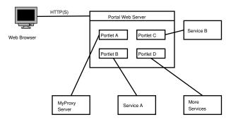
Figure 5. Complex client – portal Web server structure.
