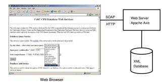
Figure 2. Structure of the CFD query Web service.
