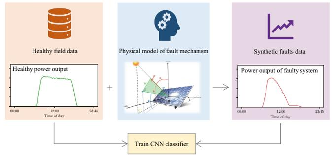
Fig. 1. Training scheme of the physics-informed deep learning model for fault detection in solar power plants. Healthy field data (left) is augmented using a physics-based fault simulator (middle) to generate synthetic fault data (right). The augmented data is used to train a deep CNN classifier.
