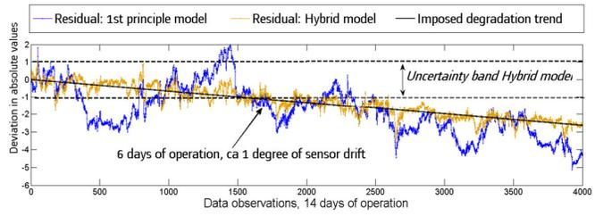
Figure 12: Residual evaluation of the first principle model and hybrid model. The hybrid PIML approach (orange) is able to follow the degradation (black) much more accurately than the pure physical model (blue).
