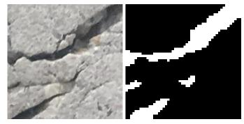
(a) Original image from data set (b) Result of *q*-means on downcontaining cracks scaled image
