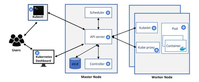
Fig. 1: A brief overview of Kubernetes. Kubernetes users interact with the installation using the Kubernetes dashboard and 'kubectl'. The purpose of master node is to maintain the desired cluster state and manage worker nodes. Worker nodes are used to run containerized applications inside the pod.
