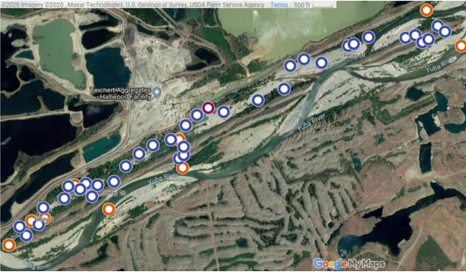
Fig. 1. Map of the network deployed in November 2018 through May 2019 on the lower Yuba River. The orange nodes are the sensor nodes, the blue nodes are the relay nodes, and the maroon node is the gateway node. This map was generated using Google My Maps.
