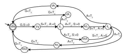
Figure 2: Fragment of data acquisition system modeled through a timed automaton.
