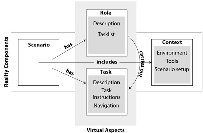
Fig. 3. The general setup behind the triggering concept in this project, including the virtual aspects of tasks and roles, as well as the reality components of the scenario and real-life context including the environment, setup and used tools.
