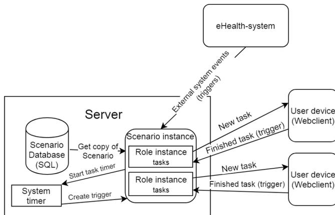
Fig. 7. The architecture of the server-client, displaying functionality within the server, and interactions between server, client and eHealth-systems.
