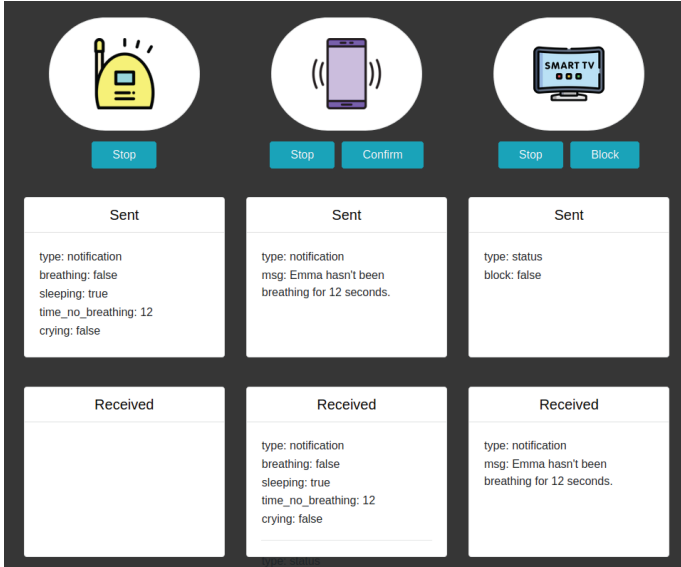
Fig. 3: Interface of Baby Monitor simulation using broker
