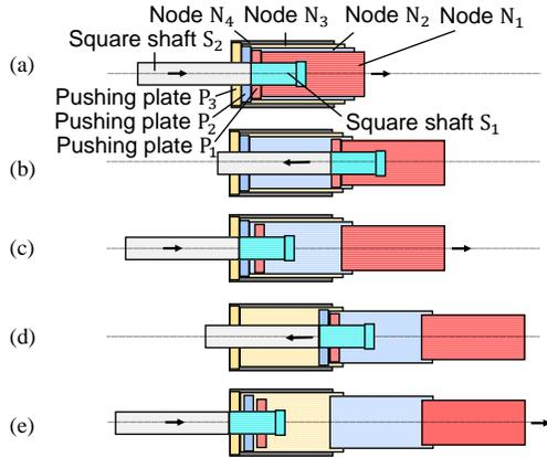
Fig. 3. Concept image of reciprocating mechanism
