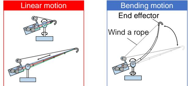
Fig. 1. Concept of tendon-driven elastic telescopic arm
