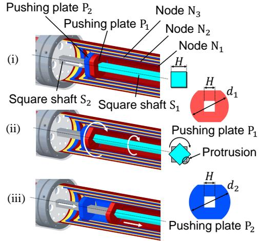
Fig. 4. Selection method. The shape of the pushing plate is chamfered for convenience of explanation.
