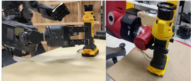
Fig. 1. Grasping of a DEWALT cutout tool with known 3D model by (a) HRP-5P humanoid on the left and (b) Sawyer arm on the right.
