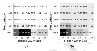
Fig. 7: Parameter optimization for learning the model space parameters  $W_{out}$  for 1000 samples (a) and 7500 samples (b).
