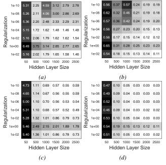
Fig. 6: Optmization for torque and payload prediction for a single ELM model. The figure shows the cross validation results for torque prediction (left) of joint 2 to 5 for 1000 samples (a) and 7500 samples (c). In addition the cross validation results for payload prediction (right) are shown in (b) for 1000 samples and (d) for 7500 samples.
