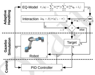
Fig. 3: Proposed control architecture for equilibrium based assistive handling modes on lightweight robots. Equilibrium model (1), estimation of prediction error (2), posture update based on prediction error (3), threshold based activation of posture update (4), desired joint angles (5), position controller (6) and robot simulator (7).
