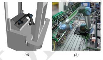
Fig. 1: Simulation setup (a) and constrained application area (b) of the UR5 industrial lightweight robot. High flexibility in the workplace design of the robot as well as individual configuration leads, e.g. cables, protective shields leads to uncertainty in robot model.
