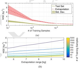
Fig. 8: Evaluation of the payload prediction. (a) shows the MSE on the test set in relation of the number of samples from the training (green) and extrapolation (red). (b) evaluation of the extrapolation capabilities.
