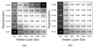
Fig. 4: Results for parameter optimization with no payload. Given values represent the mean euclidean error of joint 2 to 5 for five-fold cross validation on (a) N=1000 and (b) N=7500 random selected samples of the recorded data set.
