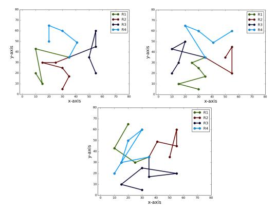
Figure 5.5: Routes produced by the optimal (left; makespan 109.4), pIA (middle; makespan 121) and sIA (right; makespan 149) methods for a Solomon instance with 16 tasks and four robots.
