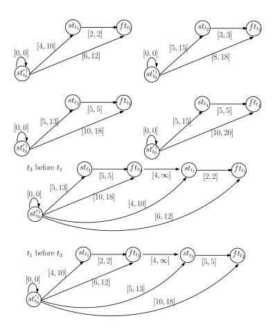
Figure 4.4: (Top four) STN for robot  $r_1$  after the insertion of the individual tasks  $t_1, t_2, t_3$ , and  $t_4$ . (Bottom two) STN for robot  $r_1$  after the insertion of task  $t_3$  after task  $t_1$  was allocated. Constraints between  $t_0$  and tasks' start and finish times account for robot travel to the task (e.g. in [4,10], 4 is the time it takes  $r_1$  to reach  $t_1$ ).
