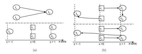
Figure 5.4: A simple worst-case example demonstrating the vulnerability of the iterated auction to certain mistakes. In (a), the example is defined by three tasks with precedence graph shown on the top of the figure, and task locations and initial robot locations are shown below. In (b), the optimal allocation is shown on top, while the iterated auction allocation (for any prioritization) is shown on the bottom.
