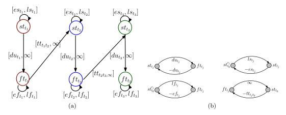
Figure 4.2: (a) Example of an STN for the tasks assigned to a robot. The STN has the time points, duration, and travel time constraints for three tasks assigned to the robot. (b) Transforming time window constraints into STN taking into account duration constraints (top left), start time constraints (top right) finish constraint (bottom left) and travel separation constraint (bottom right)
