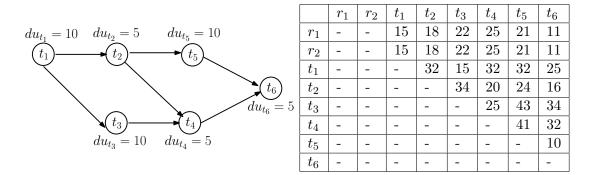
Figure 5.3: (Left) Precedence graph for 6 tasks with tasks' durations also included. (Right) Robot to task and task to task distance matrix for 6 tasks and 2 robots. Distances are symmetric and equivalent to travel time.
