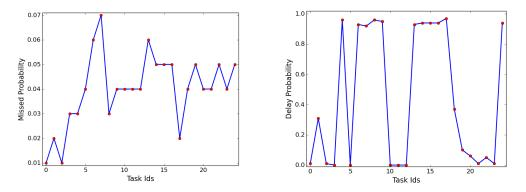
Figure 6.10: (Left) Probability of task failure and (Right) probability of task delay both measured as frequencies over the number of simulations for 25 tasks and 10 robots.
