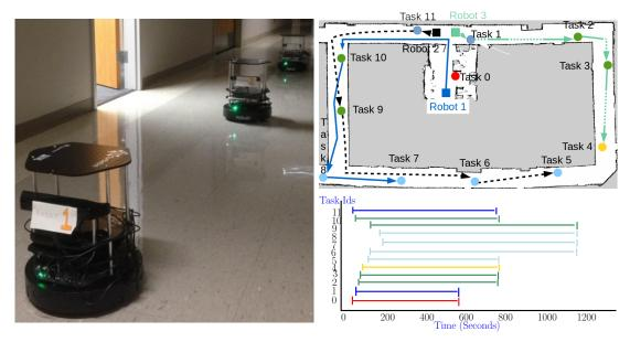
Figure 1.1: (Left) Our testbed with three turtlebots. (Right-Top) A task allocation problem instance with turtlebots and 12 tasks in a room and corridor scenario. Tasks are represented as circles and robots as squares. Tasks' colors encode precedence constraints: red precedes darker blue tasks, darker blue precedes green and lighter blue, green precedes yellow. (Right-Bottom) Tasks' time windows, each task lasts 20 seconds.
