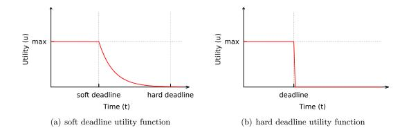
Figure 2.1: Utility of soft deadlines vs. hard deadlines. The maximum utility is earned before the deadline. An exponentially decaying utility can be gained if the task finishes between the soft and hard deadlines (case (a)). No utility is gained after the (hard) deadline (case (b)).
