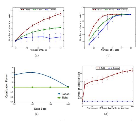
Figure 4.6: Offline experiment 1: (a) Number of tasks allocated for dataset 1 (having 20-100 tasks with 10 robots), and (b) for dataset 2 (having 100 tasks with 5-50 robots). (c) Approximation factor from optimal for small data sets with 5, 10, 15 and 20 tasks and 2, 3, 4, and 5 robots, respectively. The optimal is based on MIP 4.1. Online experiment: (d) Number of tasks allocated to 10 robots. 100 tasks arrive dynamically in batches of 1,5,10-100.
