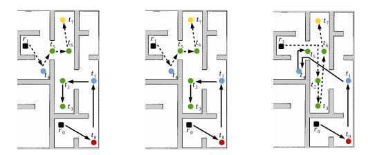
Figure 6.3: Routes produced by the optimal (left; makespan 2.87, distance 96.88), pIA (middle; makespan 3.06, distance 96.88) and Greedy (right; makespan 4.03, distance 154.26) methods for a data instance with 8 tasks and two robots. Makespans are measured in minutes and distances in meters. The colors represent tasks' precedence where red precedes blue, blue precedes green, which precedes yellow.
