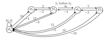
Figure 4.5: Example Distance graph for STN for  $r_1$  after the insertion of task  $t_3$  (bottom  $t_1 \prec t_3$  plot in Figure 4.4).
