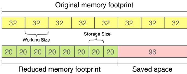
Fig. 3: Variable data-width buffer, from 32 down-to 20 bits.
