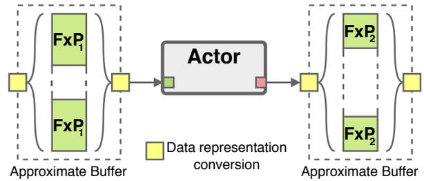
Fig. 4: Variable data-width buffer with FxP representation.
