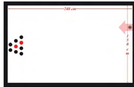
Figure 2. Experimental setup, the arena consisting of informed robots (indicated by red circles) and naïve robots (indicated by black circles), and the target at the top right side of arena
