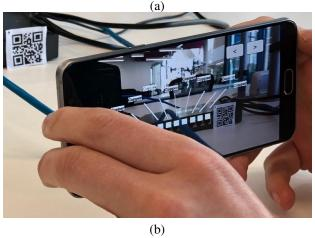
Fig. 3. An example of the (a) output of the AR App and (b) the close-up view of the App working with a 8-port network switch.
