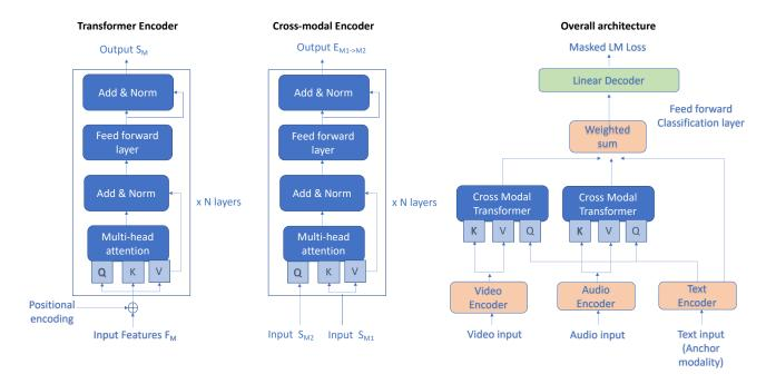
**Fig. 1**. Cross-modal transformer based self-supervised learning architecture. The figure shows the self-attention based transformer encoder layers, the cross-modal attention encoder module and the overall architecture of our self-supervised model.
