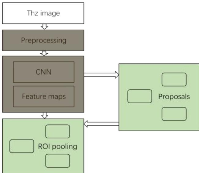
Figure 6: Object detection framework (R-PCNN) with preprocessing of THz human body security image
