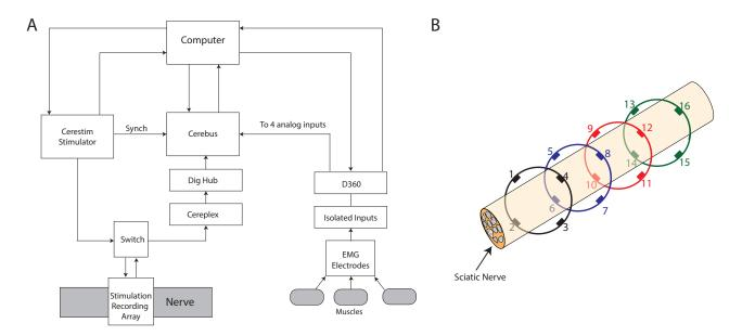
Fig. 1. A) Recording and Stimulation system setup; B) Relative positions of the electrodes in the rings within the cuff, electrodes 1, 5, 9 and 13 are on the same side of the cuff along its length and electrodes 1, 2, 3 and 4 are contained within the same ring.
