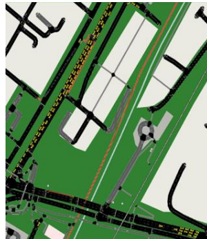
Fig. 9b: Signal alteration causes congestion at adjacent road links (1 hour later)
