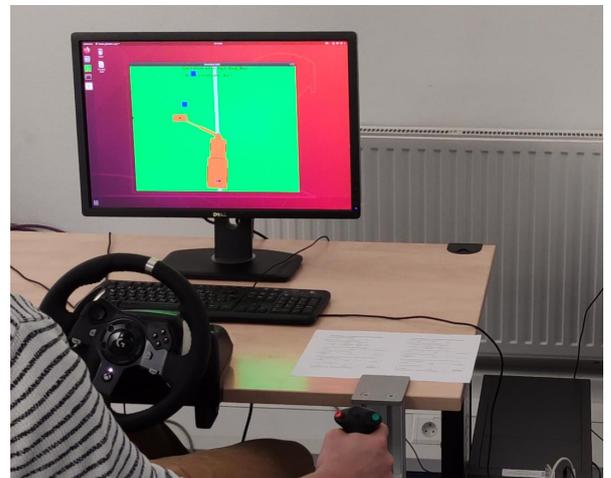
Fig. 3: An image of the test-bench with the GUI, steering wheel and joystick (bottom right).
