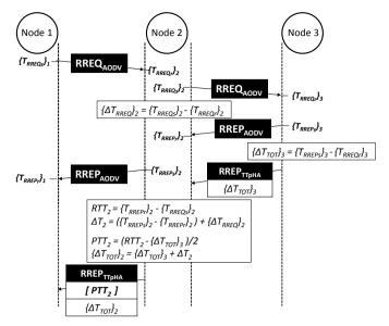
Fig. 1. The TTpHA extended AODV route discovery procedure.
