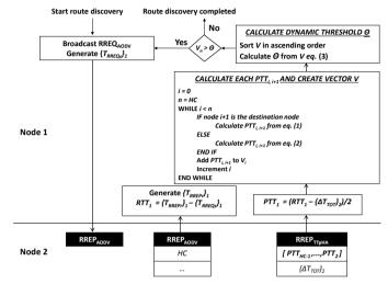
Fig. 2. Flowchart of the TTpHA algorithm at the source node (node 1)
