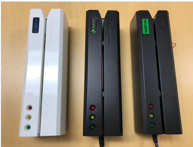
Fig. 5: The three manual card encoders we examined (from left to right): the Lanora LNR910, Osayde MSR605U, and the Misiri MSR750. Despite being sold under different brands and vendors, these devices are functionally identical.
