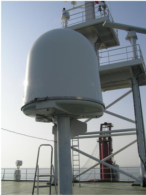
Fig. 1: A typical marine VSAT system [14].
