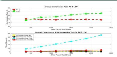
The applied techniques achieve average compression rates of 74-88% for the LZW method. If low execution times are mandatory, the AH algorithm is the best choice, achieving approximately 74% compression rate for all packet sizes.
