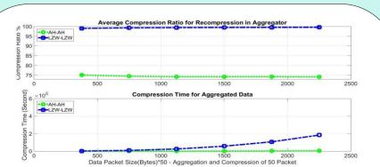
both meters and aggregator using AH (AH-AH) or LZW (LZW-LZW) It easily can be seen that the LZW approach shows a higher compression rate which is expected from Fig. 2 due to the larger data packet size after aggregation.
