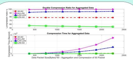
We applied the compression algorithm inside the aggregator on compressed packets received from 50 smart meters. The results shows that the best compression ratios are obtained when LZW techniques are applied in the aggregator after AH compression on smart meter.
