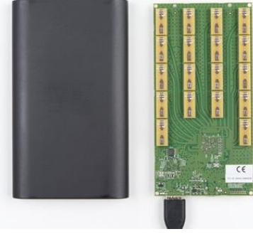
Figure 4. Walabot hardware antenna array
