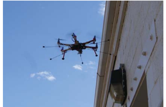
Fig. 1. The Hexrotor is performing an inspection task. Note the rotor axes are not parallel
