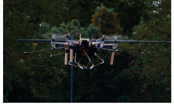
Fig. 6. Hexrotor flying with manipulator.
