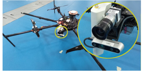
Fig. 2: Platform with camera detail.
