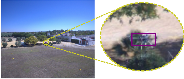
Fig. 5: Long-Range Detection: sample full frame with UAV detection detail.
